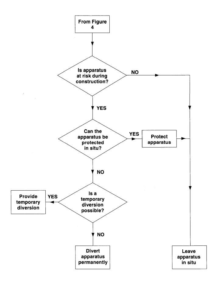
FIGURE 3 APPARATUS AT RISK DURING CONSTRUCTION
